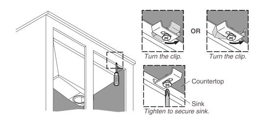
□ Rotate the clips and tighten the screws (not provided) to secure the sink to the countertop.
