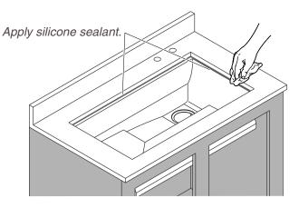
☐ Apply silicone sealant. Immediately wipe away any excess.
