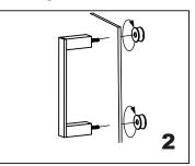
Screw in the fixing brackets into the handle bolts.
