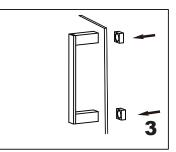
Add the end caps on the fixing brackets, make sure the set screws holes in the bottom.
