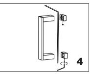
Fix the set screws on the end caps,tighten it to avoid loose from fixing brackets.
