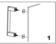
Install the handle A (bolt) through the glass holes, make sure the rubber gaskets are between handle&glass.
