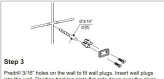
Predriil 3/16" holes on the wall to fit wall plugs. Insert wall plugs into the wall. Position backing plate flat side down over the plugs and install screws.
