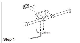
Loosen the set screw on the accessory and remove the backing plate. Position the accessory against the wall and mark outline with pencil.
