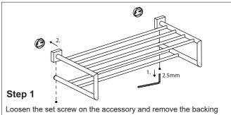
Loosen the set screw on the accessory and remove the backing plates. Position the accessory against the wall and mark outline with pencil.
